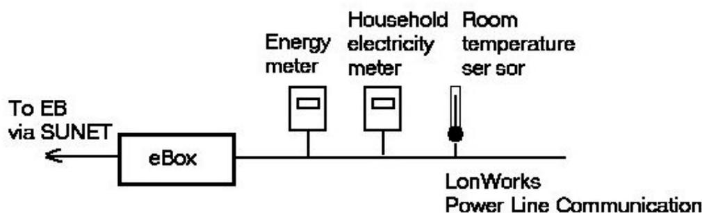
Figure 6.3. Measurement design of the Energy Barometer demonstrator
