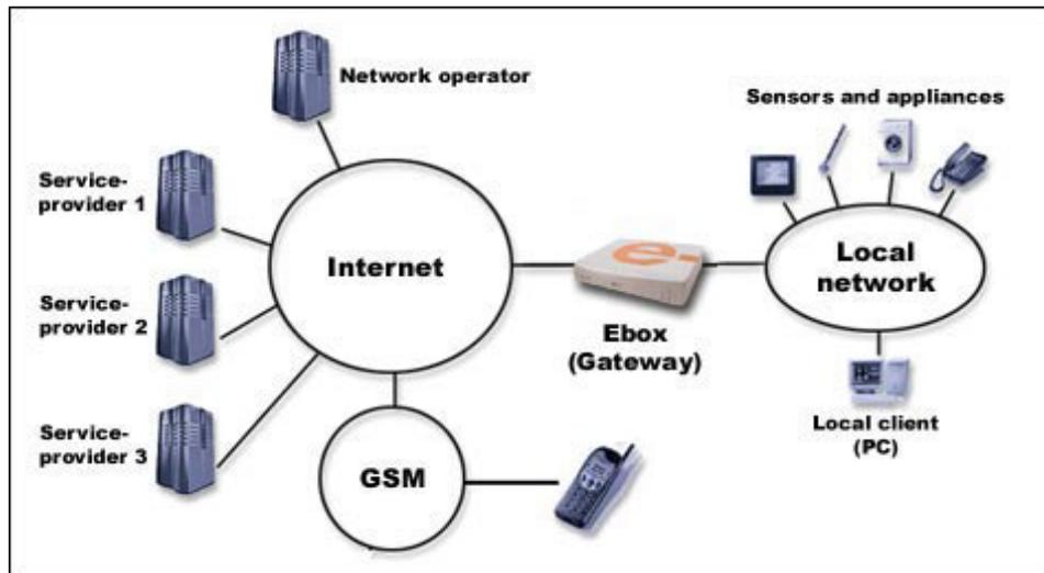
Figure 6:1. Network of an electronic service system
