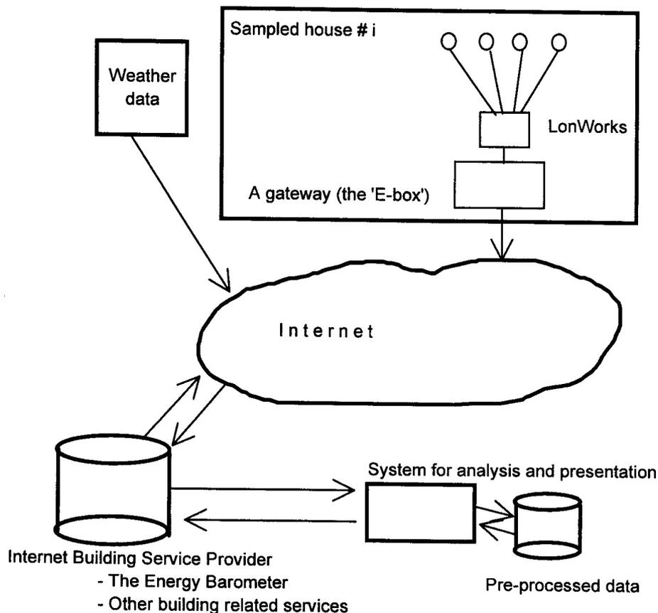
Figure 6.2. Structure of the Energy Barometer system
